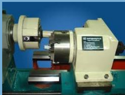
Polygon Turning Attachment
